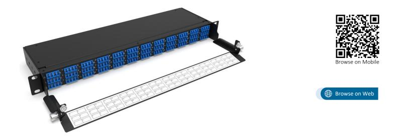
Nexconec High Density MTP/MPO to LC breakout Patch Panel offers an expandable deployment, for implementations in 40G/100G networks, in the meantime, providing greater protection to the installed patch cords in main, horizontal and equipment area of data center. Up to 144 Fibers in only 1U space.
