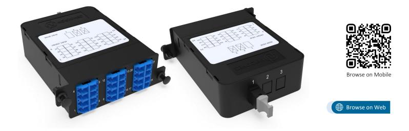
NEXCONEC® HD MPO transition cassettes are pre-terminated modules MPO-LC fanouts that are suitable for up to 100G applications to interconnect backbone with discrete connections. The HD cassettes are designed to easily plug into NEXCONEC HD 1U 4 slot chassis and each chassis can populate up to 96F. The cassettes eliminate the need for splicing reducing costs. The MPO and single ferrule connectors are available in Standard and Elite versions to cater to the customer's power budget requirements.
