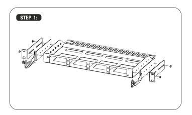
Assemble the door mounting bracket and side bracket with the screws supplied in the zip lock bag as below pic show.
