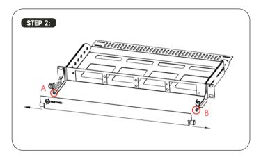
Assemble front door: pull the spring plungers outside and then plug it into the holes A & B.
