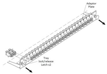
2. The tray can be positioned at 45-degree angle to carry out further assembling of fiber optic products if needed.
