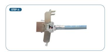
Fit the wire retention cap to the rear of the jack (it will only fit one way round) and push it down to seat the wires in to the IDC slots.
