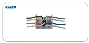
Pass the wires through the hole in the rear of the wire retention cap and dress the wires in to the appropriate coloured slots following the preferred wiring configuration.
