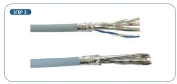
If using U/FTP cable fold the foil of one of the pairs back and wrap it around the outside of the cable sheath with the silver surface on the outside.
