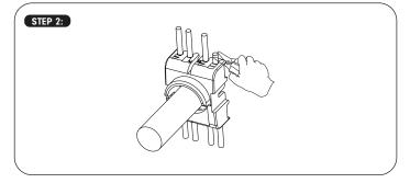
Insert the cable into the termination cap and fan out all four twisted pairs. Following the instruction of the color coded wire position printed on the termination cap, put wires into the slots and make sure the wires are in the proper slot. Trim the exceeded wires.
