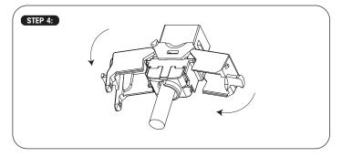
Press the punching wings, punch the termination cap into the keystone.
