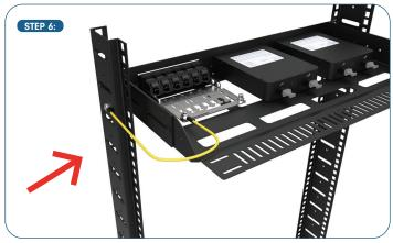
For shielded keystone jacks, attach the ground wire to the rack.
