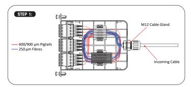
Splice the  $1^{st}$  set 12 rainbow pigtails as above picture shown (Please cut the  $600/900\mu m$  pigtails according to the real installation).
