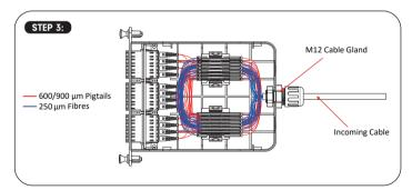
Above picture is the cassette fully spliced with 2 sets pigtails.
