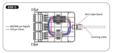
Splice the  $2^{nd}$  set 12 rainbow pigtails as above picture shown (Please cut the  $600/900\mu m$  pigtails according to the real installation).
