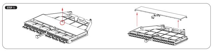
Use two fingers to pick the middle area of lid (as shown above in pic-1) and lift up to easy remove the lid from module to access patching adapters.
