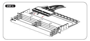
Insert patching module from rear side of the panel & keep enough margin of patchcords in the rear side to make sure easy movement of the module.
