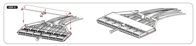
Insert back the lid by matching lid flange (1) with module holes, then match middle part (2) and hold middle area with a thumb and then match lid flange (3) with module holes to make easy and perfect fit.
