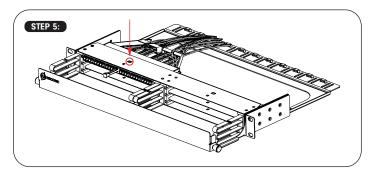
Rotate the push/pull tab of the module into lock position to restrict its movement.
