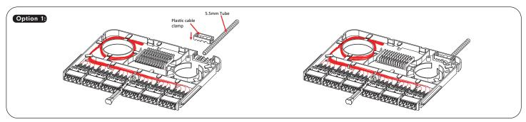
For the use of Bluelite conduit/ 5.5mm diameter tube, clamp the incoming fibers tube directly by pressing on top of the plastic clamp until it locks.
