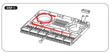
Remove the plastic cable clamp and choose the cable/tube slot from one of the 4 slots as per installation requirements. (Picture shown above)
