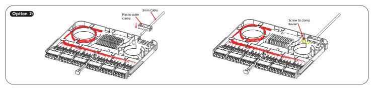
For 3mm diameter cables you can insert 1 or 2 cables of 3mm as shown above. Once the cables are into position press on top of the plastic clamp until it locks. If the incoming cable contains aramid yarn, you can screw that into the hole for additional strain relief.
