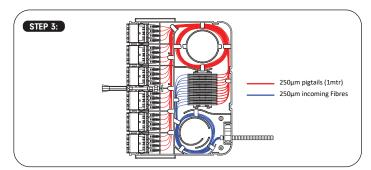
Please refer to above for the fiber routing of incoming cables to the splice holders. The fibers of the incoming cables are 250 microns and the fan out length recommended is 200mm.
