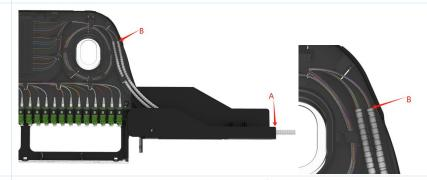
Insert the 250um bare fibers around the spools and coil it counter clockwise, we recommend at least 3 coils.
