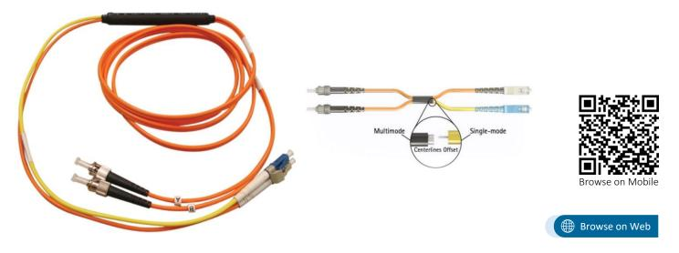
NEXCONEC<sup>®</sup> Mode Conditioning Patch Cord is used for Gigabit Ethernet applications where Gigabit routers and switches are installed into existing multimode cable units. These patch cords mainly prevent the differential mode delay, by setting the launch from the single-mode to be offset from the center of the multimode fiber.
