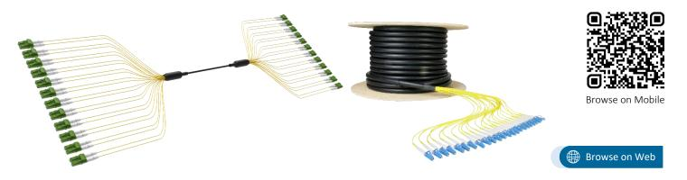
NEXCONEC® Indoor/Outdoor Preterms offers quick and cost-effective installation for interbuilding, LAN or Campus wide network. These indoor/outdoor preterms are made of single gel filled PBT tubes and each tube consists of 12 or 24, 250µm optical fibers, the tubes are surrounded with longitudinally applied E-glass non-metallic strength members, Corrugated Steel Tube (CST) armor and UV resistant LSZH or PE jacket.
