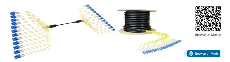
These NEXCONEC® Indoor/Outdoor Preterms are made of Microcore Flex Armored cable, contains 12 of 250µm optical fibers in a micro tube, accommodated in the helical flex armored tube and surrounded by E-glass, Kevlar, water blocking yarn and UV resistant LSZH outer jacket.
