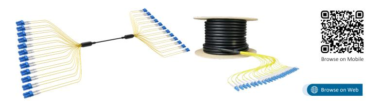
The NEXCONEC® Outdoor Flex Armored Preterms are made of single loose tube, which consists of 12 (250μm) optical fibers, aramid strength member in the steel armored helical tube and surrounded with metal braiding, Kevlar and PU outer jacket for high crush resistance in the outdoor applications.
